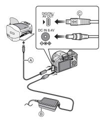
(A): USB connection cable (supplied)(B): AC adaptor (DMW-AC7PP; optional)
